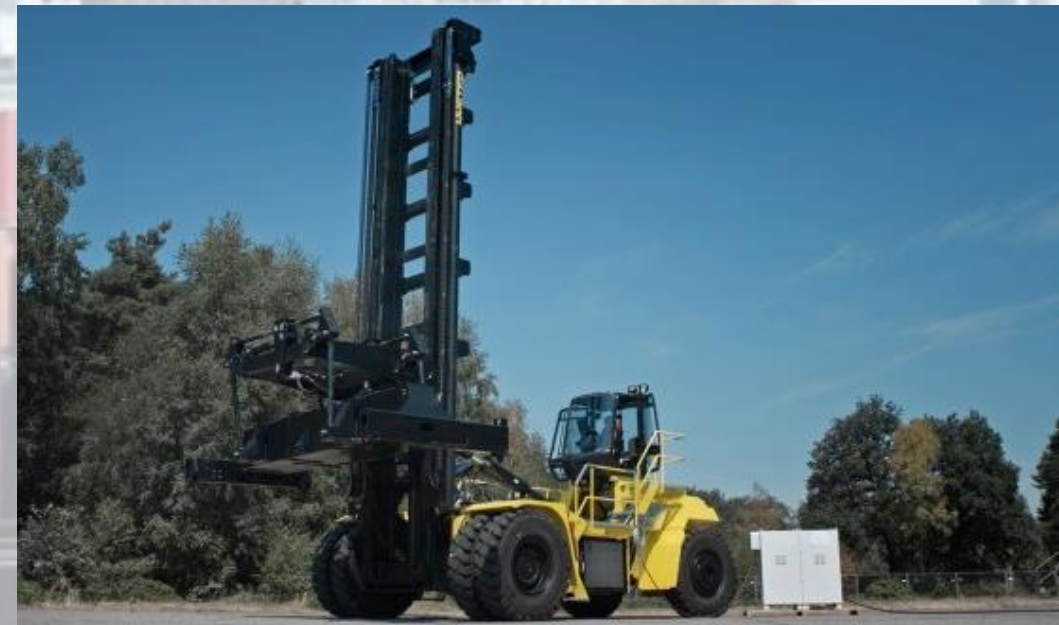
Photo of the hybrid fuel cell-battery-powered container handler under development by Hyster for use in California. Source: Hyster
